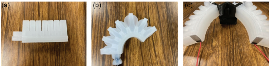
FIGURE 3.10 Developed robot hand that contains two soft silicone fingers: (a) developed soft robot finger and (b) curved form when filled with air. (c) Soft robot hand equipped with two soft robot fingers and conductive cloth is embedded in the fingertip.
