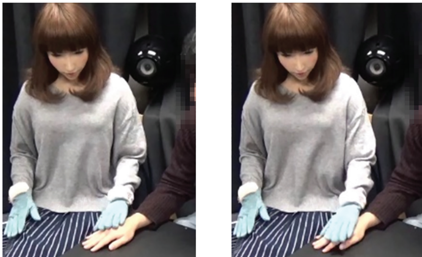
FIGURE 12.1 ERICA's hand touch behaviors (left: using her palm, right: using her fingers).
