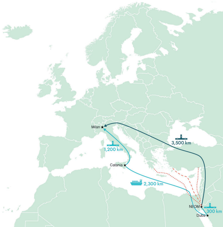
FIGURE 8.16 Comparison of shipping and pipelines as hydrogen transport methods from Saudi Arabia to southeast Europe.
