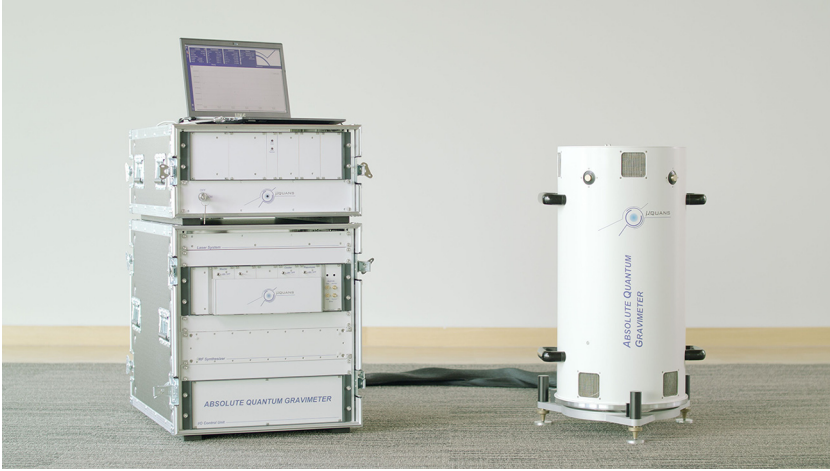
FIG. 2.8 – Photograph of the atomic gravimeter marketed by the company Muquans. On the left, the laser bench and the control electronics. On the right, the drop chamber in which the cold atoms are in free fall.
