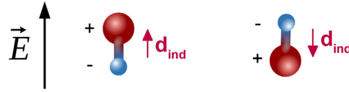
FIG. 7.8 – When electric field \vec{E} is applied in the laboratory, electric dipolar molecules acquire on average an induced electric dipole moment d_{\text{ind}} , along the electric field. The most electronegative atom, i.e. the one which tends to attract the shared electrons of the molecule, is represented by a blue sphere, and the least electronegative by a red sphere. We thus associate a net charge + on the red sphere and - on the blue sphere. This defines the orientation of the induced electric dipole moment, from the - charge to the + charge. The value of this moment is positive if it is directed in the same direction as the field (left molecule), and negative if it is directed in the opposite direction (right molecule).
