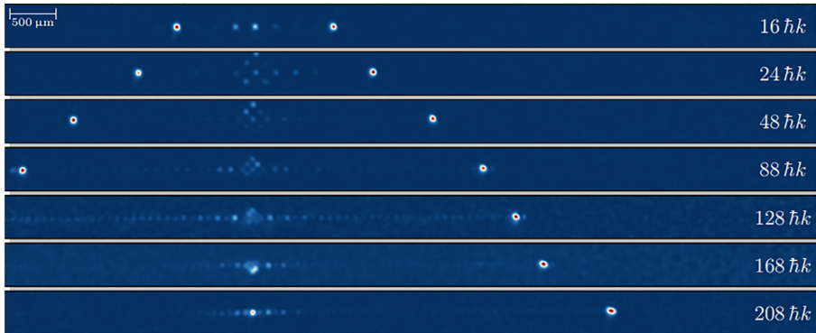
FIG. 2.9 – Spatial separation of wave packets after different large momentum transfer beamsplitters. The greater the momentum transfer, the greater the separation of the wave packets. The atoms are detected here by absorption imaging after a period of free flight after their interaction with the beamsplitters: they are then illuminated with a laser beam, the intensity of which is absorbed where the atoms are located. (Courtesy of Sven Abend, Leibniz University of Hanover).
