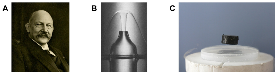
FIG. 4.1 – (A) Heike Kamerlingh Onnes (1853–1916) was the first physicist to cool helium to liquefaction temperature. He was awarded the Nobel Prize in Physics in 1913 for his work on cryogenics. (B) At low temperatures, liquid helium becomes superfluid : it loses all viscosity and flows without resistance, giving rise to unusual phenomena, such as the fountain effect shown here. (C) Similarly, at sufficiently low temperatures, some materials become superconducting : their electrical resistance strictly vanishes. A magnet placed on a superconductor can levitate above the superconductor. These phenomena have forged our understanding of the physics of collective effects of quantum origin. But other phenomena, now observed for 35 years, remain mysterious, such as superconductivity at a high critical temperature.
