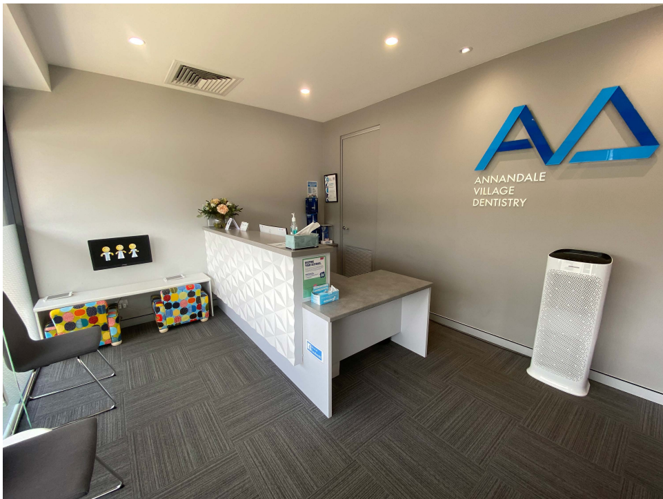
Figure 2.1 An inclusive reception desk for use by people of different heights or mobility.
