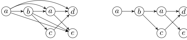
Figure 3.1: The Dependence Graph (left) and Hasse Diagram (right) for the trace [abcaed] according to the trace monoid \mathbb{M}(A, Z) over the alphabet A = \{a, b, c, d, e\} and independencies Z = \{(a, c), (c, a), (b, d), (d, b), (d, e), (e, d)\} .
