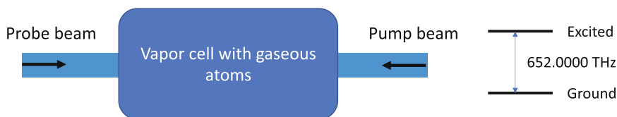
Fig. 5.2 Saturated absorption spectroscopy needs two laser beams: a probe beam and a pump beam. Not pictured is the photodiode with which we monitor the transmission of the probe beam
