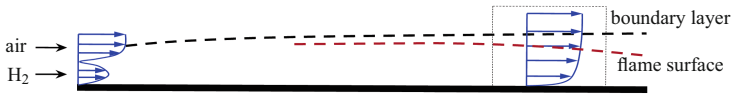
Fig. 1. Diagram of the simulated flow configuration. The area within the dotted rectangle represents the fully developed reacting boundary layer flow, investigated in the present paper.
