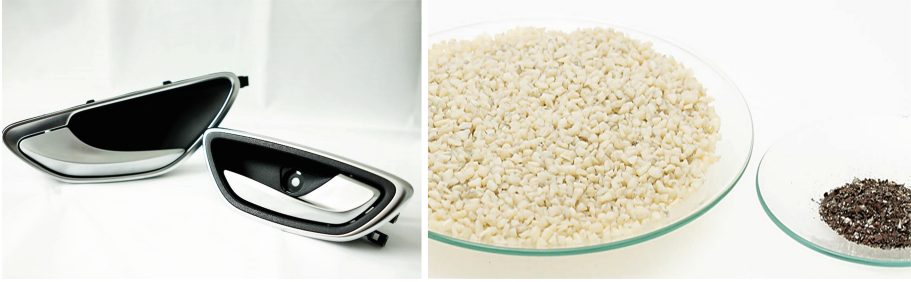
Fig. 2. Left: Plated applications in the interior; right: separated polymer and metal fraction after the recycling process
