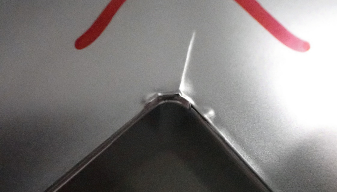
Fig. 6. Cracks in the coating after climate change test (DBL1665 AKLV 42 Cycles)
