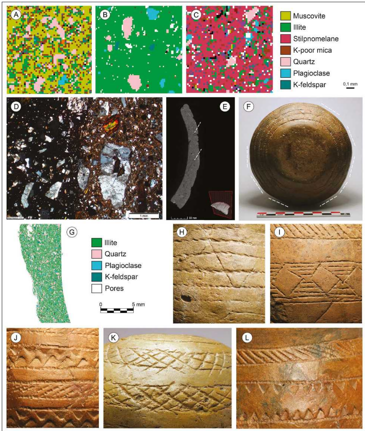
Figure 5: Synthesis of the Bell Beaker pottery tradition for the 'Petit-Chasseur' necropolis. QEMSCAN® mineralogical map of ceramic matrix: A) muscovitic groundmass; B) illitic groundmass; C) stilpnomelane groundmass. Temper material: D) granite particles in the ceramic paste. Forming techniques: E) coiling junctions visible through micro-computed tomography; F) small facets characteristic of the beating technique; G) dense fabric and extremely fine porosities (QEMSCAN® mineralogical map of PC1 MXI Gob.1). Decorating techniques: H) Z-twisted cord impression; I) indented tool impression; J) indented tool and stamp combination. Finishing treatments: K) and L) burnishing.
