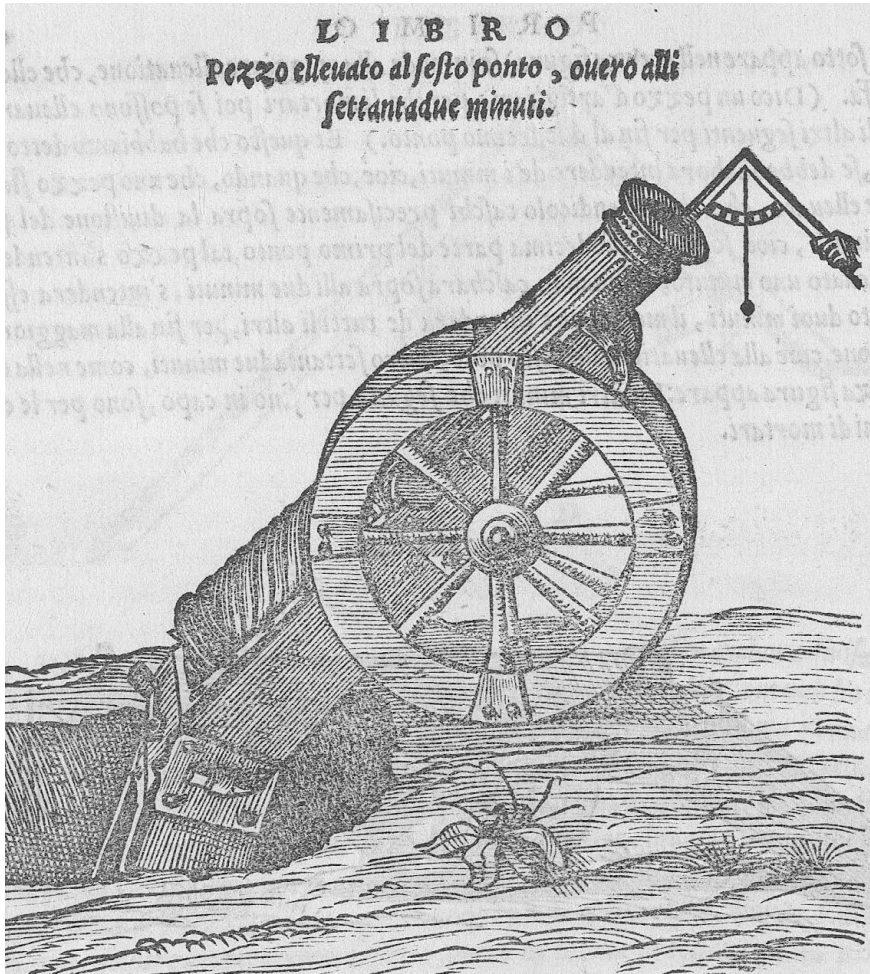
FIGURE 6.18 Artillery piece positioned for indirect fire. (Nicolo Tartaglia, Quesiti et Inventioni Diverse (1554), p. 6v. Courtesy of ETH-Bibliothek, Zurich)
