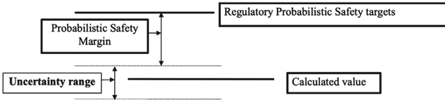
Fig. 2.3 The logical basis of a probabilistic safety margin. Published with kind permission of the IAEA, Source and copyright holder: International Atomic Energy Agency, Safety Margins of Operating Reactors Analysis of Uncertainties and Implications for Decision Making, IAEA-TECDOC-1332, IAEA, Vienna (2003). All rights reserved
