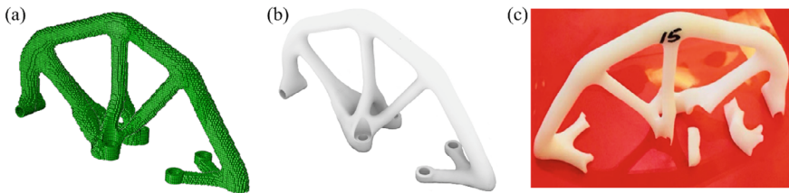
Fig. 3.11 Final optimized hinge arm for the load case of an upward load: a finite element model; b smoothed model; c 3D printed prototype after mechanical loading test (reprinted from Xiong et al. 2021, licensed under CC-BY 4.0)
