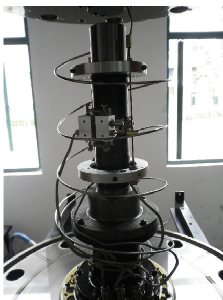
(c) Installation method of extensometers
