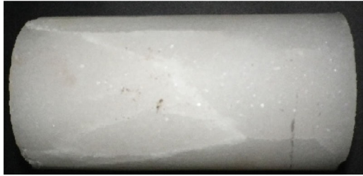
(a) Uniaxial compression with no dynamic disturbance
