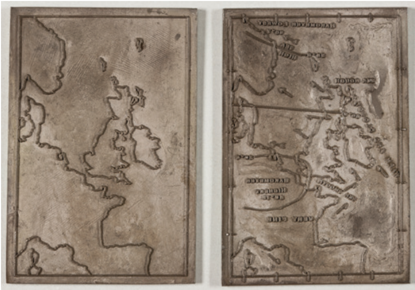
Figure 10.1 Prototype printing plate for a newspaper weather map, created by Francis Galton. LDUGC-026. Courtesy of the UCL Eugenics Collection.
