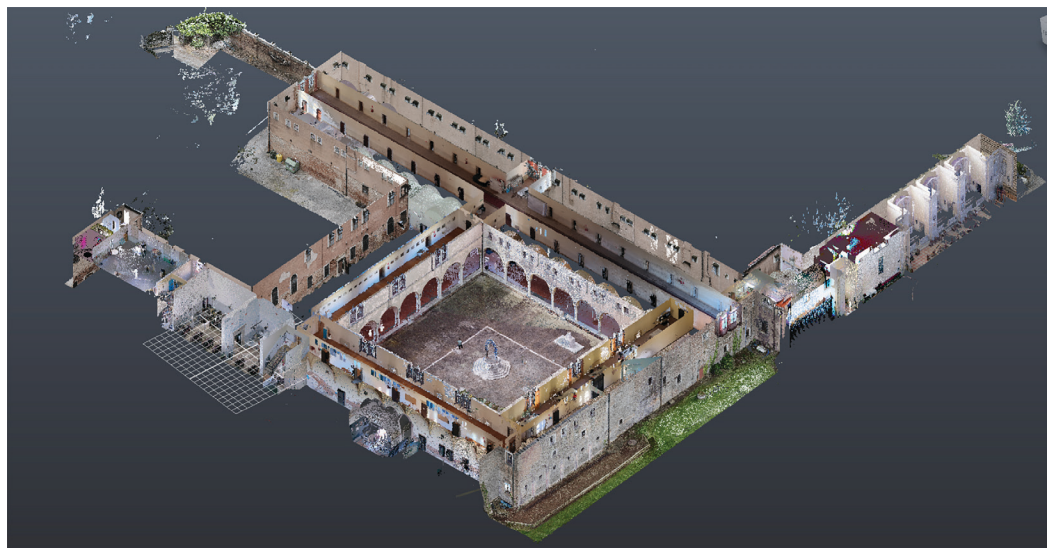
Fig. 7. Total point cloud resulting from the integrated survey in sectioned axonometry. (elaboration by authors).
