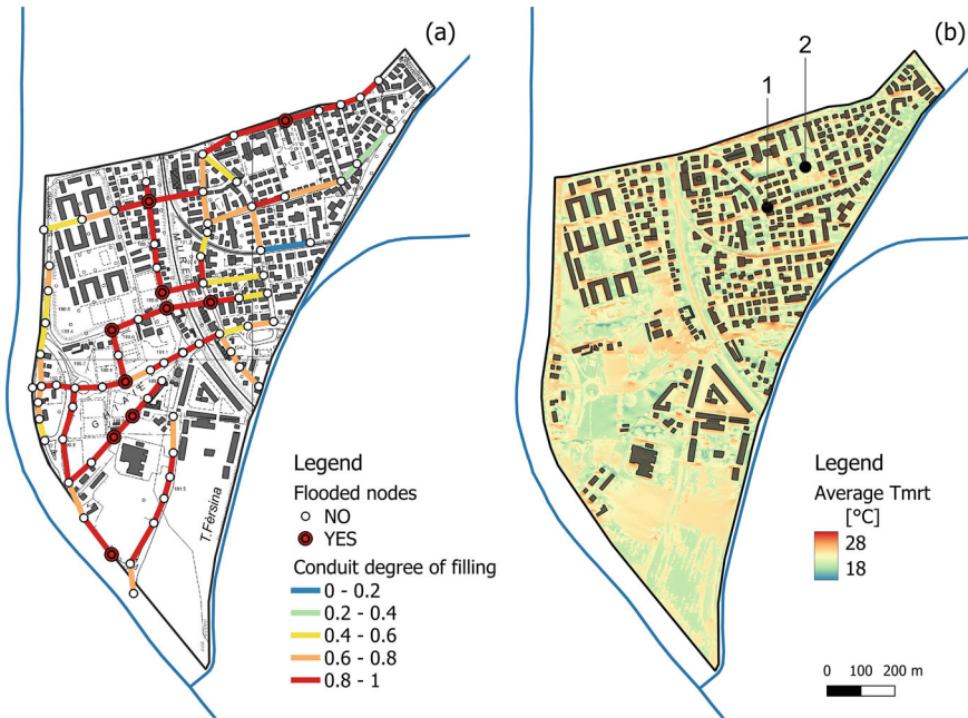
Fig. 2 Spatial distribution of flooded nodes and conduit degree of filling of the drainage network (a), and average simulated mean radiant temperature within the study area in summer 2023 (b)
