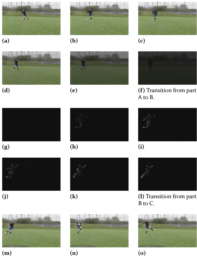
Figure 4.17.: Extension of video summary system: integration of video and audio effects. Video was divided into three parts: (A) beginning of video clip to heel strike, (B) heel strike to ball contact, and (C) ball contact to end of video clip.
