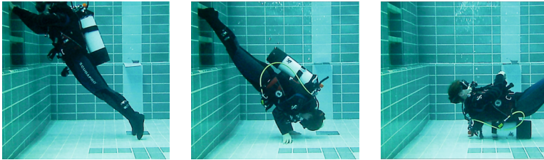
Figure 13: Examples of resting poses for the determination of the upper body orientation with an IMU attached to the chest. © 2015 IEEE, printed with permission [P1].
