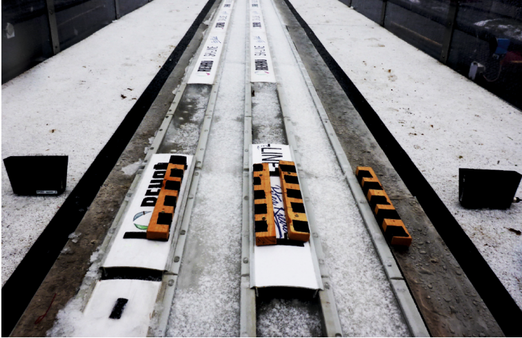
Figure 21: Take-off platform with magnetic gate and light barrier system. When an athlete passed the construction, four permanent magnets (two for the left, two for the right ski) produced a distinct peak in the magnetometer signal. Simultaneously, the light barrier was triggered. © 2017 ACM, printed with permission [P5].
