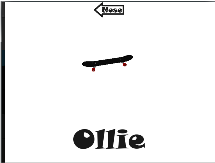
Figure 38: Main screen of the implemented GUI. The skateboard is continuously visualized in its current orientation by means of a 3D-animation. As soon the classification pipeline provides the detected trick, its name is visualized in addition. © 2017 Elsevier, printed with permission [P9].
