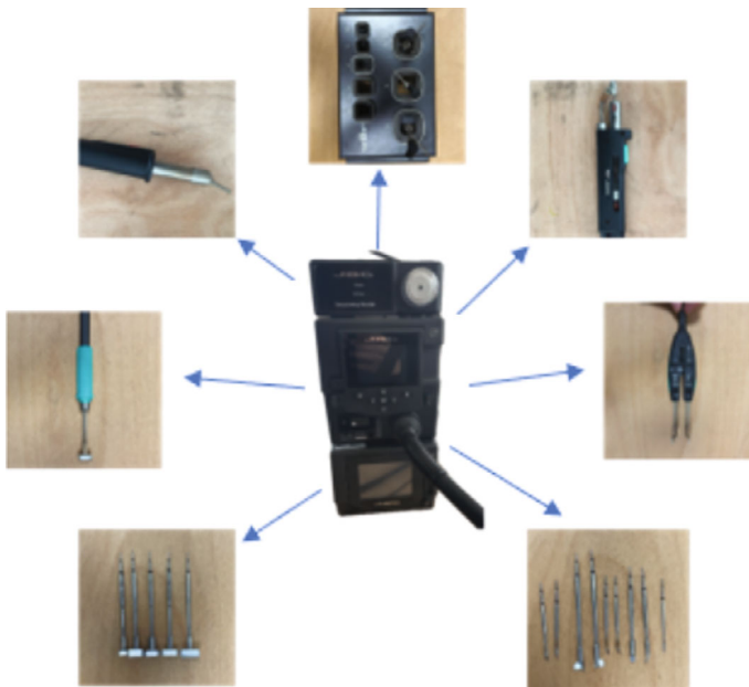
Fig. 2 The precision rework tools used during manual disassembly tests
