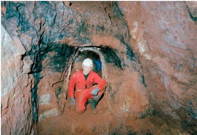
Figure 7.6: Photograph of a chamber on the fault in the Cobalt Mine at Alderley Edge with a round shaft in the floor. The black coating is cobaltian wad (photograph by Paul Deakin).
