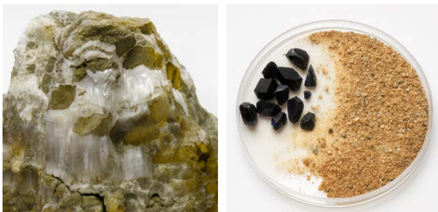
Figure 8.1: Photographs of (left) cobalt alum in veins in host rock; (right) dark blue glass made from the granular artificially produced pigment (right side of Petri dish).
