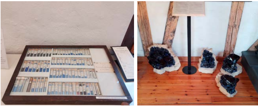
Figure 4.2: Photograph of (left) examples from the collection of raw materials and products (smalt, slig, oxide, etc.) of the Blaafarveværket mine in Modum, Norway; (right) crucibles for smalt making with glass attached, held at the Blaafarveværket museum.
