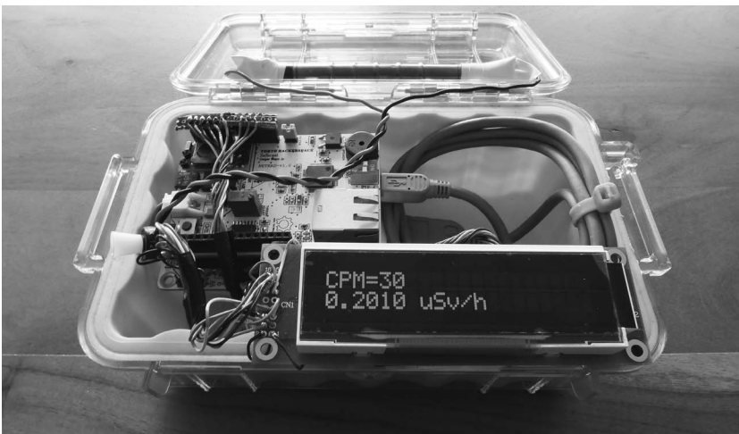
FIGURE 5.1 Early Geiger counter prototype, Akiba’s NetRAD
