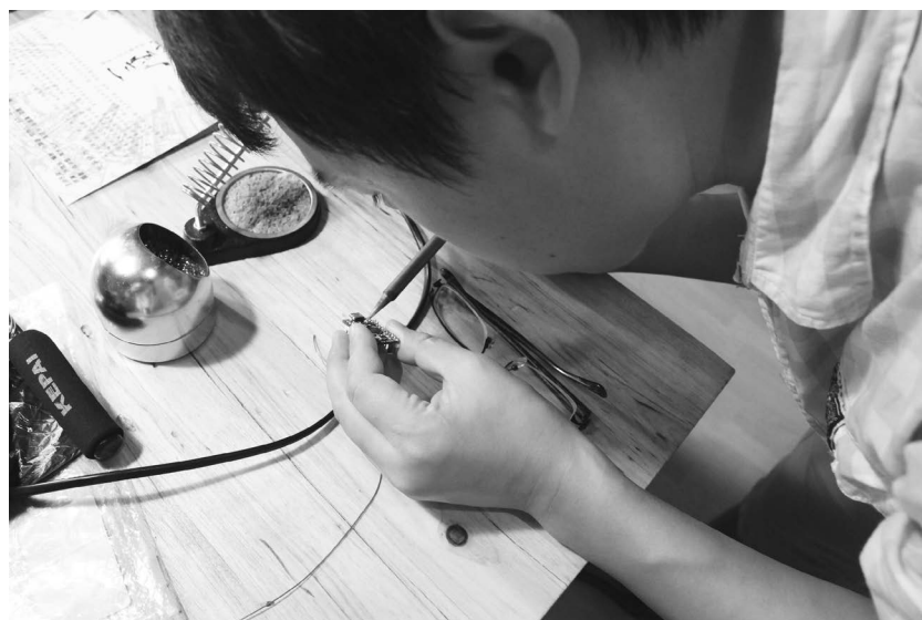
FIGURE 3.2 Atommann fixes a broken micro-USB connector on a circuit board
