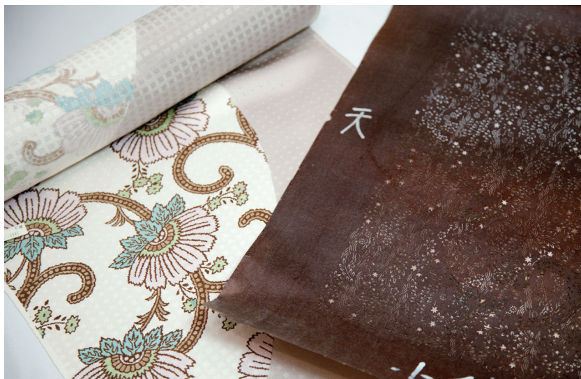
Photo 12: A kata-yuzen stencil and kata-yuzen fabric. Since its origin in the Edo period, hand-drawn yuzen has undergone periodic transformations, using stencils in the Meiji period and jet printing in the modern era. Photo: Yunosuke Kawabe
