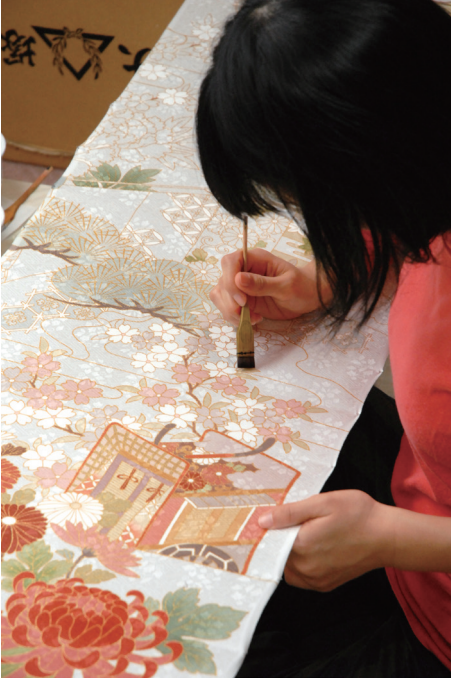
Photo 1: Applying colors: one step in the yuzen dyeing process. The craftsperson carefully mixes dyes to create the best colors and painstakingly applies them by hand.
