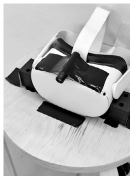
Fig. 3: Custom setup of a VR headset with mounted laser pointer for exact directional calibration
