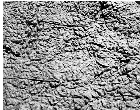
Fig. 6: Malm limestone, chemical-biological weathering, etched by plant roots; detailed view
