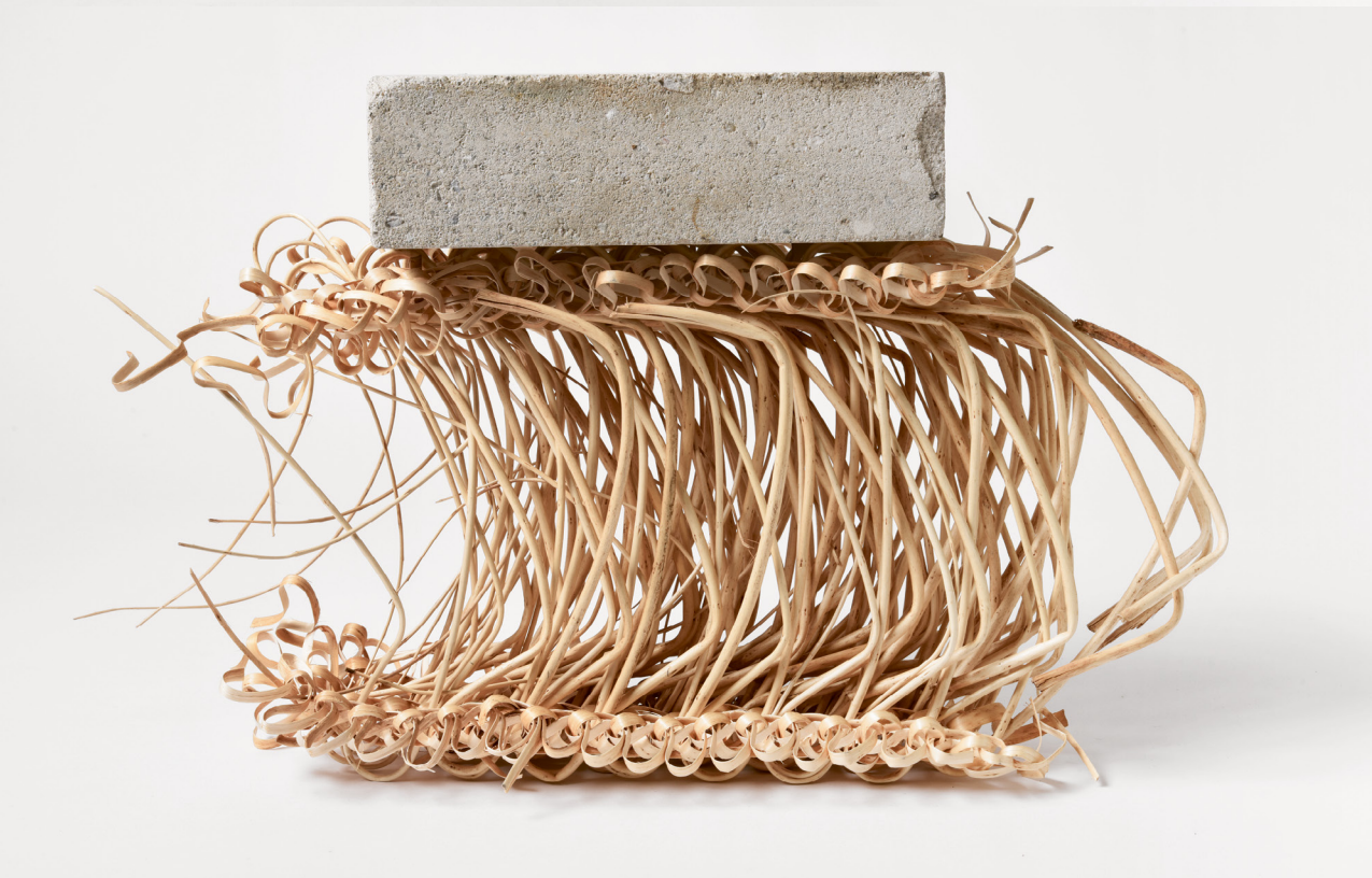
Fig. 19: Structural Textiles : The use of different materials programs the elasticity and stability of a structure, ranging from flexible and responsive (a, b) to structurally solid (c)
