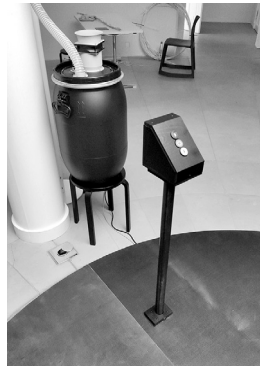
Fig. 5: A physical control station for the Virtual Elevator platform—later replaced by a virtual avatar interface to allow greater freedom of movement with material samples, cloud formations, and dynamic virtual objects
