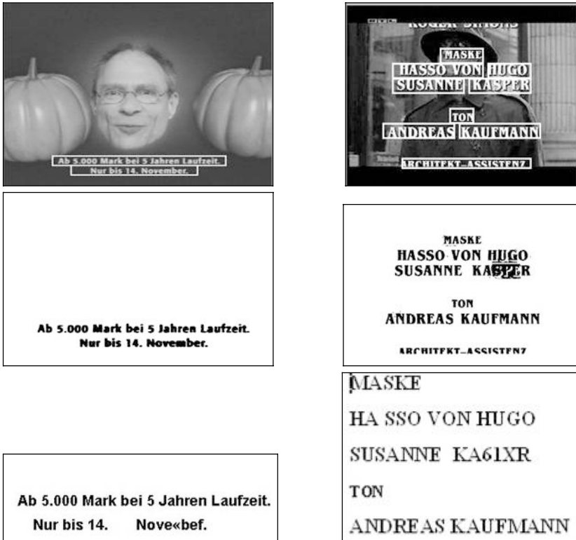
Figure 3: The images on the top row show the result of text localization. The middle row depicts the results of the text segmentation process, in which the background has been removed and the text has been marked black. In the last row, the result of the recognition software (OCR) is shown.
