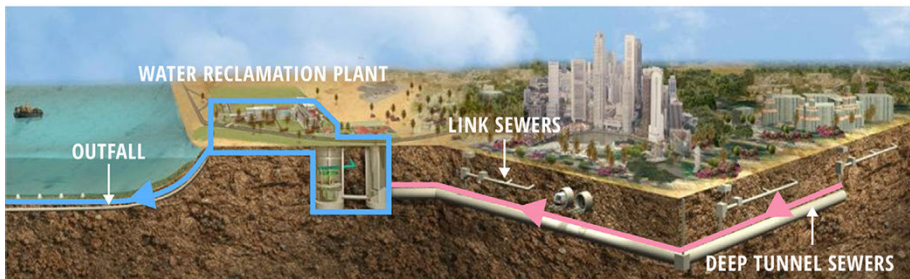
54. SECTION OF THE DEEP TUNNEL SEWERAGE SYSTEM
