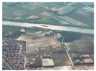
Photo 2.1 (courtesy of Frédéric Hédelin) – Aerial view of a breach caused by overtopping at St-Laurent-de-la-Salanque on the left-bank dike of the Agly, following flooding on 12-13 November 1999. The breach unfortunately appeared next to the waste-water treatment plant. Fortunately, the residents had been evacuated.
