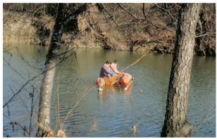
Photo 6.2 – Bathymetrical measurement using a weighted decametre on a transverse section of the River Vidourle.
