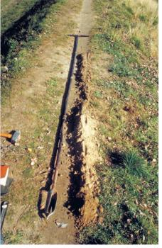
Photo 6.4 - A PDG 1000 dynamic penetrometer set Photo 6.5 - Sounding with a manual earth auger in the sandy-silt body of a Camargue dike.
