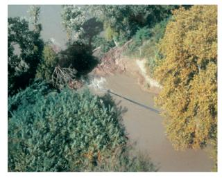
Photo 2.12 (Source: Service Navigation Rhône-Saône) – Aerial view of a Camargue dike breach that coincides with a pipe crossing.
