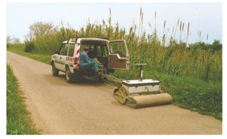
Photo 6.1 – Geophysical exploration using the radio magnetotelluric (RMT) method on the top of the Agly dike.
