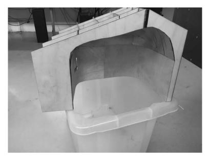
**FIGURE 5.8** A veneer model used to explore a double curvature construction. The architect noted: 'It shows how unsuccessful this idea was.'
