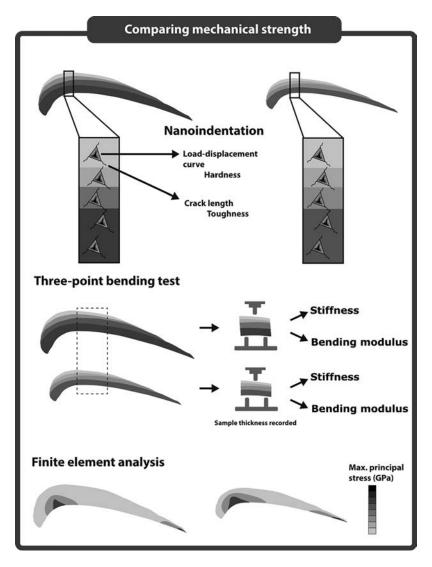
**Figure 3** Schematic representation of techniques to compare the mechanical properties of biomineralising organisms. Nanoindentation and three-point bending are two highlighted techniques for assessing mechanical properties, including hardness, elasticity, fracture toughness and stiffness of biominerals. Microindentation and nanoindentation in the combination of CT and FEA project the impact of OA on the mechanical properties of shells and skeletons during predatory attacks.
