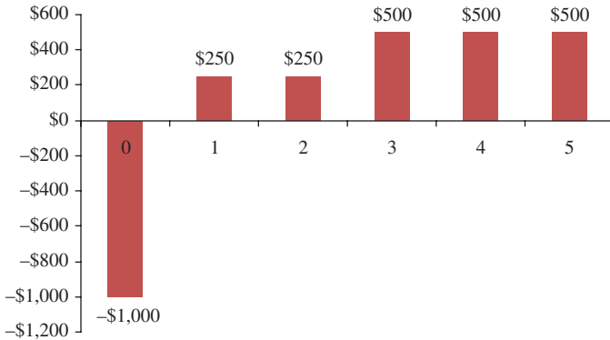
Figure A.1.2 Calculating the net present value (NPV) of a time series of costs and benefits ( i = 7\% assuming a discount rate (e.g. inflation rate) of 7% per year). For each time period, t , the value is calculated by dividing the current cost or benefit by (1 + i)^t . The NPV is then calculated by summing the value across all time periods.
