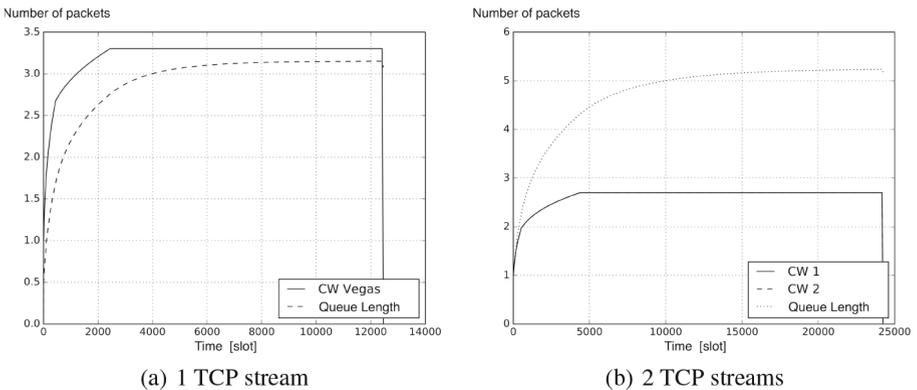
**Fig. 1.** TCP Vegas congestion window evolution — FIFO queue
