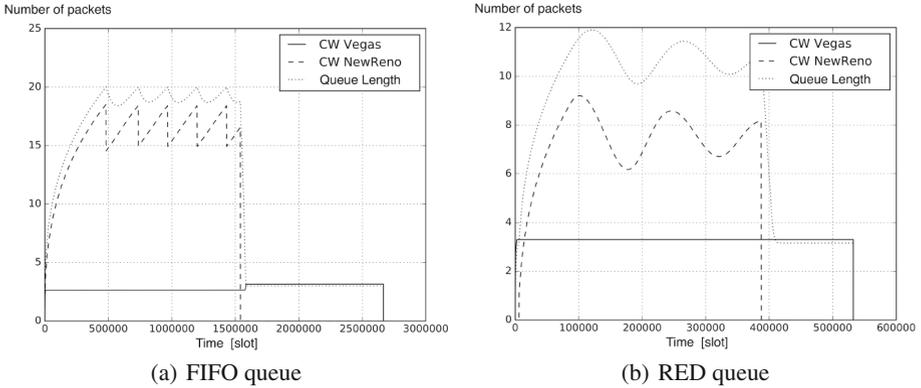
Fig. 4. TCP Vegas and NewReno congestion window evolution
