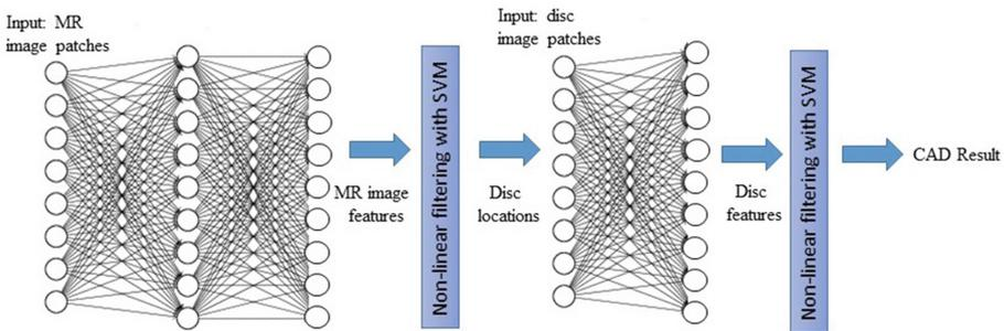
**Fig. 2.** The architecture of the system.
