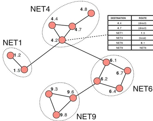
Fig. 1. Hierarchy and recursion: the routing table at node 4.2 contains information on how to reach any other node in the network.
