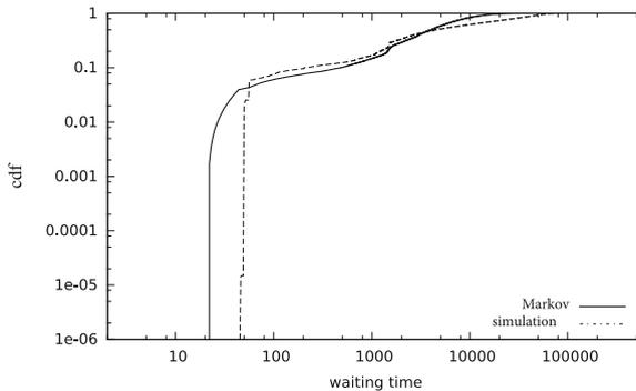
**Fig. 2.** Comparison of response time distribution given by simulation and Markov model, logarithmic time scale
