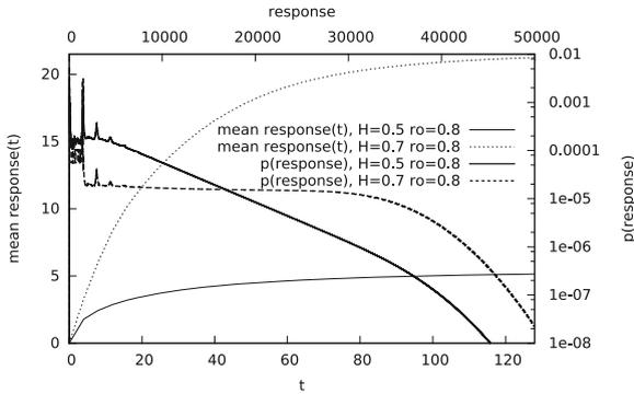
**Fig. 3.** Mean response time as a function of time and steady state distribution of response time for hyper-Erlang representation of service time distribution,  $H = 0.5, 0.7$ ,  $\rho = 0.8$
