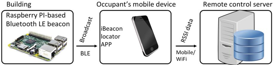
**Fig. 1.** System architecture
