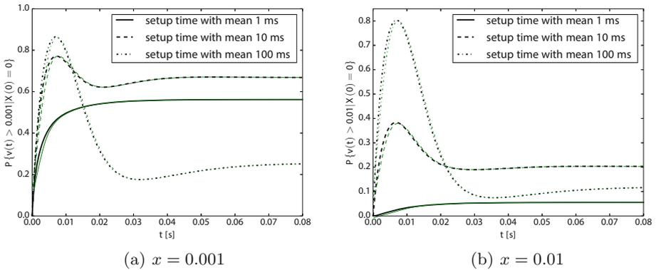
**Fig. 1.** Probabilities  $\mathbf{P}\{v(t) > x|X(0) = 0\}$  for  $x = 0.001$  (a) and  $x = 0.01$  (b), where mean setup time is equal to 1 (solid line), 10 (dashed line) and 100 (dot dashed line) ms. Bold black lines and thin green lines correspond with analytical and DES results, respectively (Color figure online)
