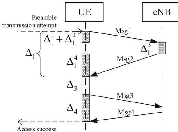
Fig. 1. Message sequence diagram for successful access
