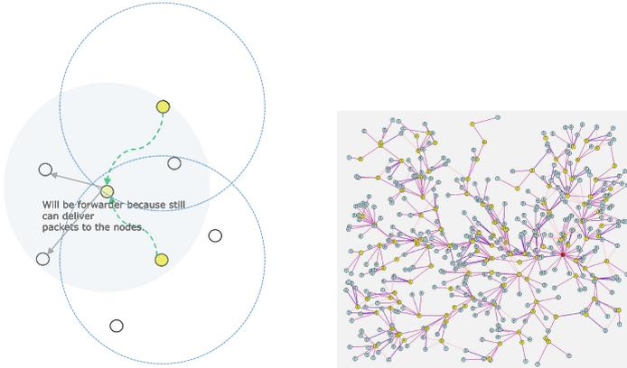
**Fig. 3.** (a) The Scalable Broadcast Algorithm used to select a forwarder node, (b) The example of logical topology created using SBA method
