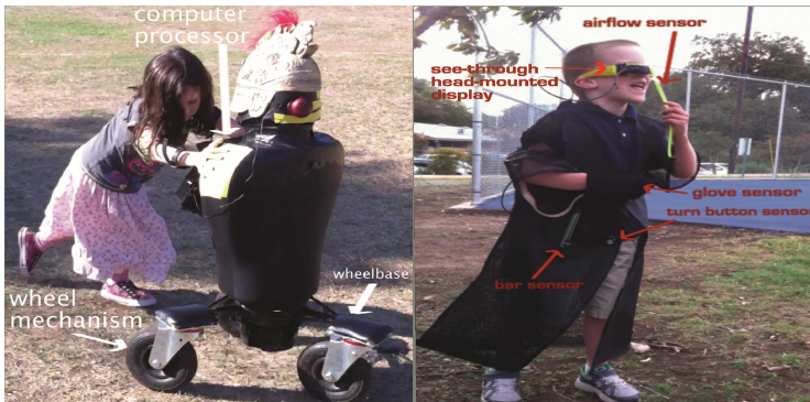
Fig. 1. Left. “Cratus”. A child pushes “Cratus” to put a game avatar into motion (visualized on the computer processor); Right. “Albert”. A child blowing air into an airflow sensor to put a game avatar into motion (visualized on a see-through head-mounted display).
