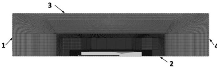
Fig. 2 Computational domain: 1—water inlet, 2—symmetry plane, 3, 4—constant pressure boundaries
