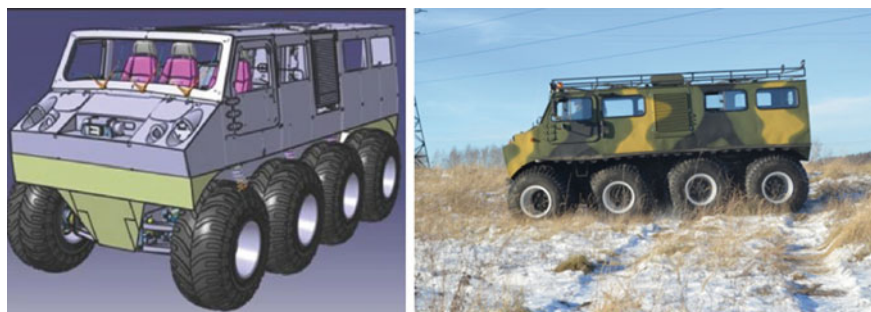
Fig. 3 General views of 3D model and experimental prototype of the produced MATV
