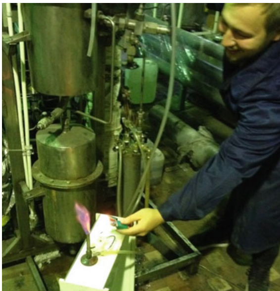
Fig. 3 The experimental verification of SCHD reaction product
