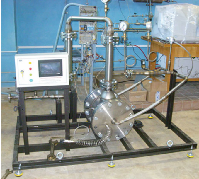
Fig. 3 Pilot installation for matrix conversion of natural gas at enhanced pressures. Input natural gas capacity up to 10 m 3 /h
