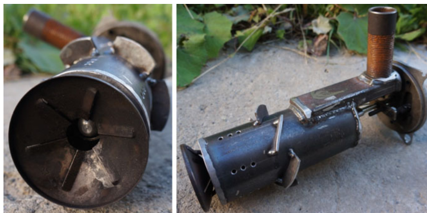
Fig. 1 Combustion head of the fuel-oil burner with a nozzle for co-combustion of gaseous fuels
