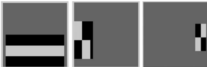
Fig. 3 Examples of Haar-like features used in the system
