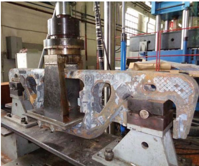
Fig. 2 Cyclic testing of the solebar
