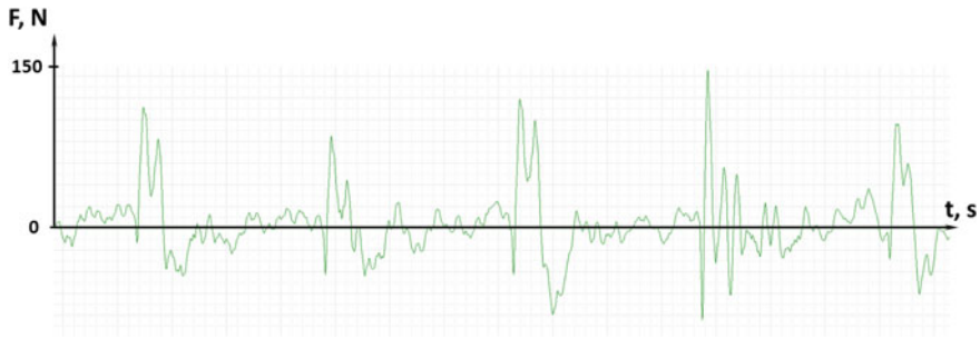
Fig. 7 Load cell record in one of the experimental runs with the pulse-detonation hydrojet operating at a frequency of 3 Hz in a water stream of 5 m/s
