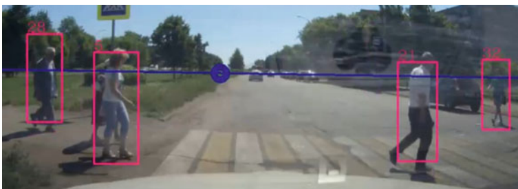
Fig. 2 Pedestrians, detected in the image (marked with rectangles), and the line of the local horizon (thickened line)
