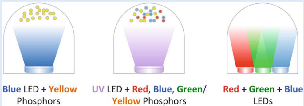
Fig. 5.16 Illustration of white light generation using phosphor method (blue/UV LEDs + phosphors) and using RGB method (Red + Green + Blue LEDs)
