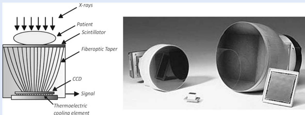
■ Fig. 13.38 In digital X-rays, a fused fiberoptic taper is used to guide the light image from a scintillator an electronic CDD detector array for processing and visualization
