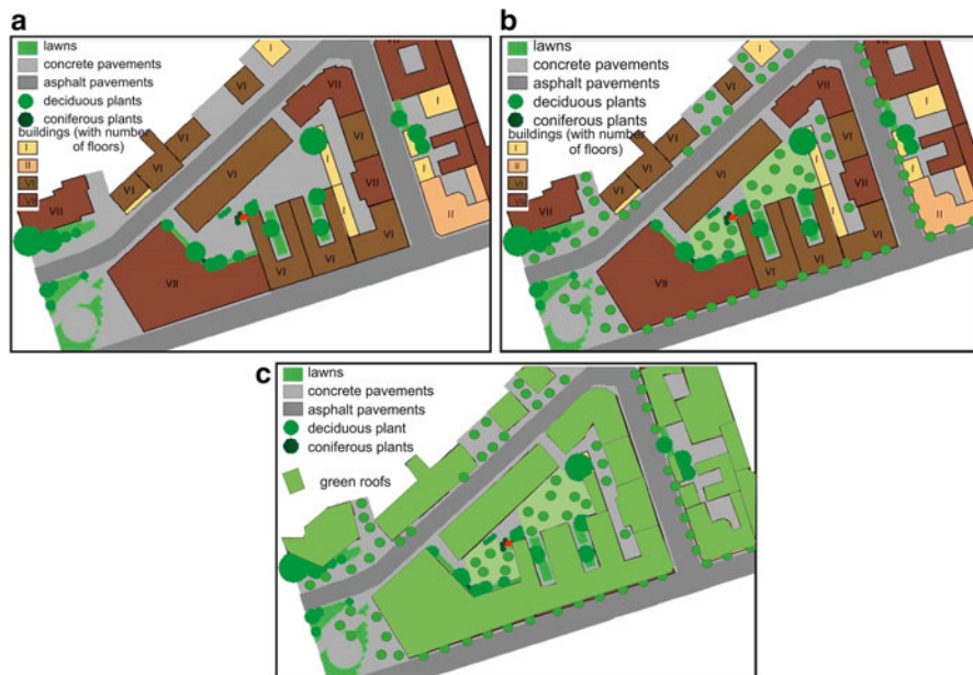
Fig. 11.7 Land cover of the Twarda district; (a) – present state, (b) – changes in land cover proposed in scenario 1 (additional trees and permeable surfaces), (c) – changes in land use proposed in scenario 2 (additional trees, permeable surfaces and green roofs)
