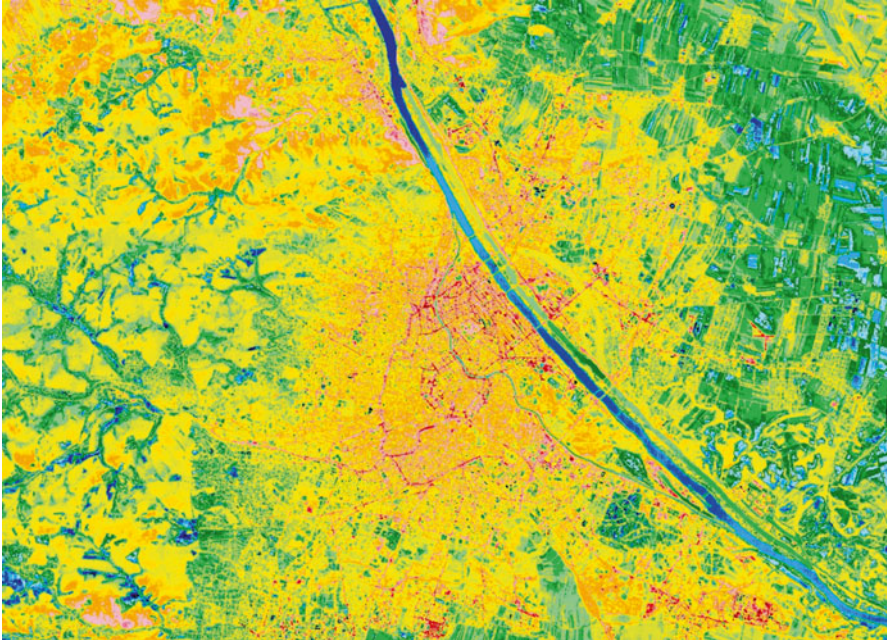
Fig. 9.1 Thermal image of Vienna and surroundings by night. There is a noticeable difference between the urban agglomeration and the cooler rural areas (Source: City of Vienna, MA 22)
