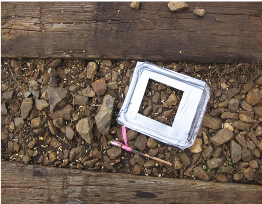
Fig. 9.2 Grain spill sampling method used on the rail bed. The sampling frame ( 10 \times 10\text{ cm}^2 ), was randomly thrown three times to estimate the mean density of wheat and barley seeds within a 5 m zone
