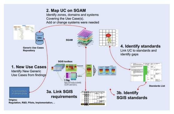
• Fig. F.1 Process to apply use cases as the basis for a standardization gap analysis under consideration of functional and security-related requirements, taken from [2]
