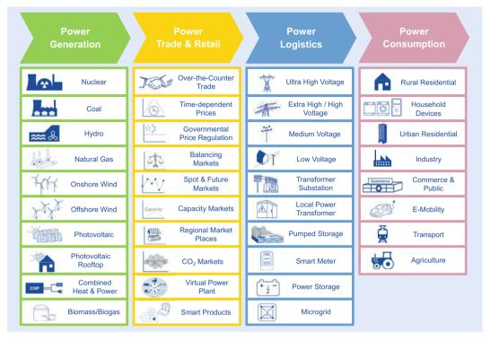
■ Fig. C.1 Power system components and market elements in the Chinese power system model
