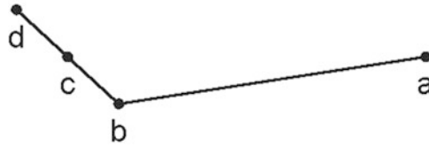
Fig. 9 A four-node graph in which nodes a and c are topologically equidistant from node b but nodes c and d are physically closer to node b
