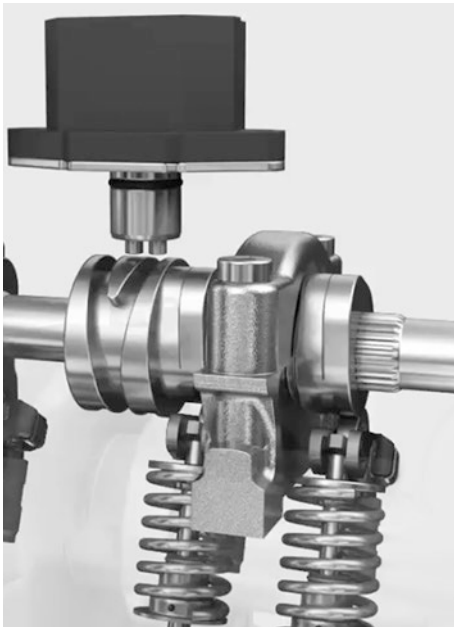
Figure 14 Two-stage cam shifting system
