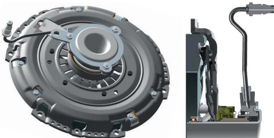
Figure 17 Travel adjusted clutch (TAC) and cover-mounted release system (CMR) with smaller cover bearing on the end of the guide sleeve [2]
