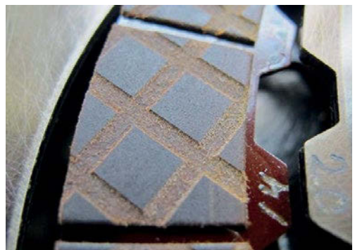
Figure 11 Endurance test with LuK friction lining: 20,000 hill starts under full load
