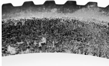
Figure 5 STC 300: Friction lining made of carbon-based composite material
