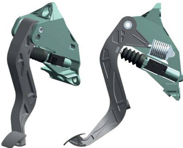
Figure 20 Pedal box for clutch operation made of plastic with integrated master cylinder and sensor
