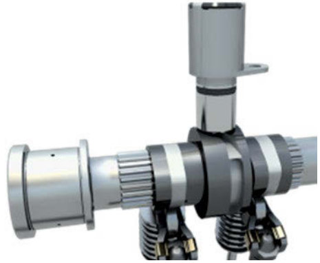
Figure 15 Three-stage cam shifting system
