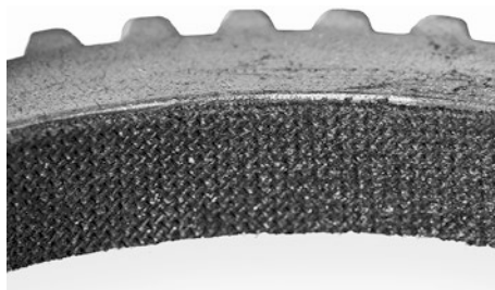
Figure 6 STC 600: Premium class carbon-based friction lining
