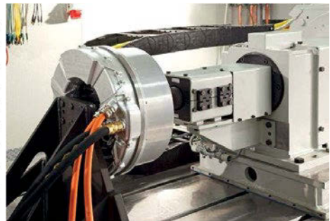
Figure 5 Test stand run with the new drive (right); efficiency data map of the electric motor with operating points from the ARTEMIS cycle (left)
