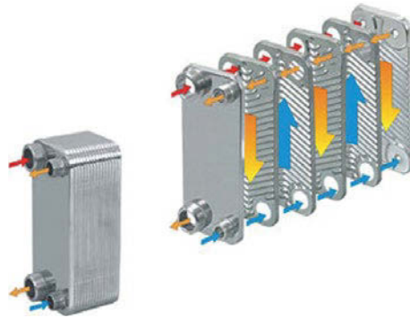
Figure 7 Design of a plate-type heat exchanger
