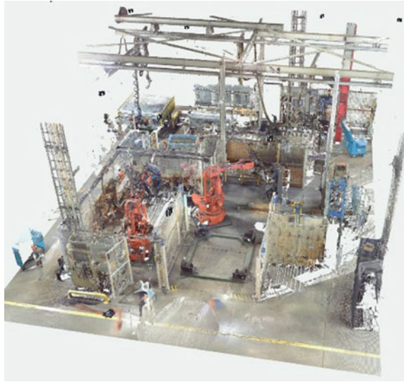
Fig. 8 3D laser scan data of the production cell used for the demonstrator
