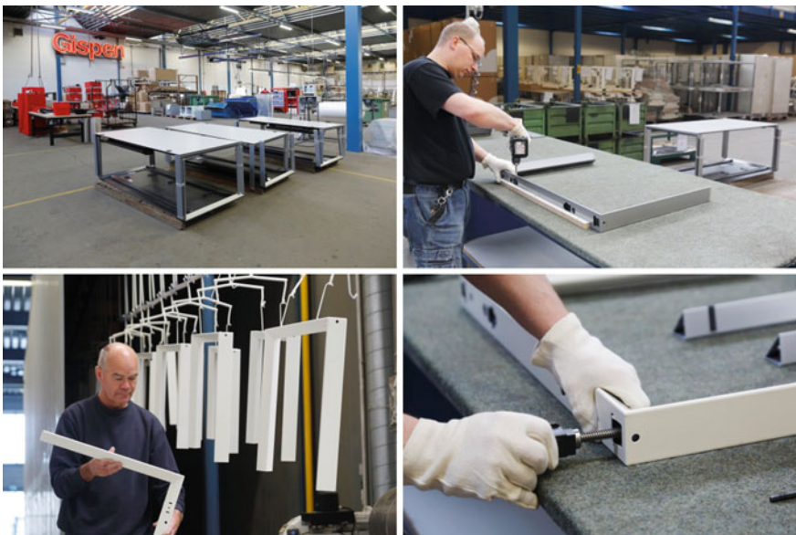
Fig. 1 Collecting, disassembly, remanufacturing and reassembling of office furniture at Gispén’s manufacturing site in Culemborg, The Netherlands
