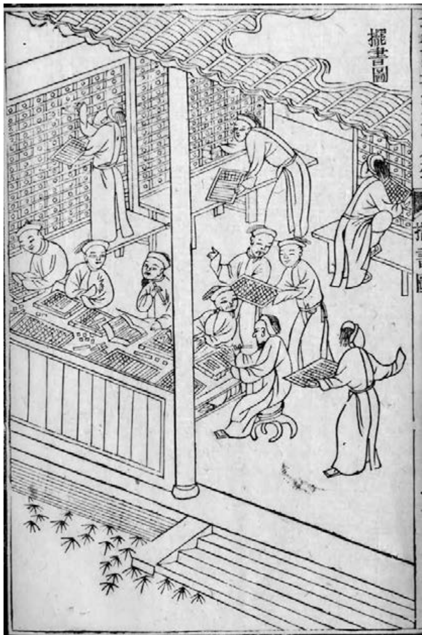
Figure 22 Type setting. This process includes selection of the types from the type cases, placing them on trays, arranging them in the right sequence, and proofing the set forms.
