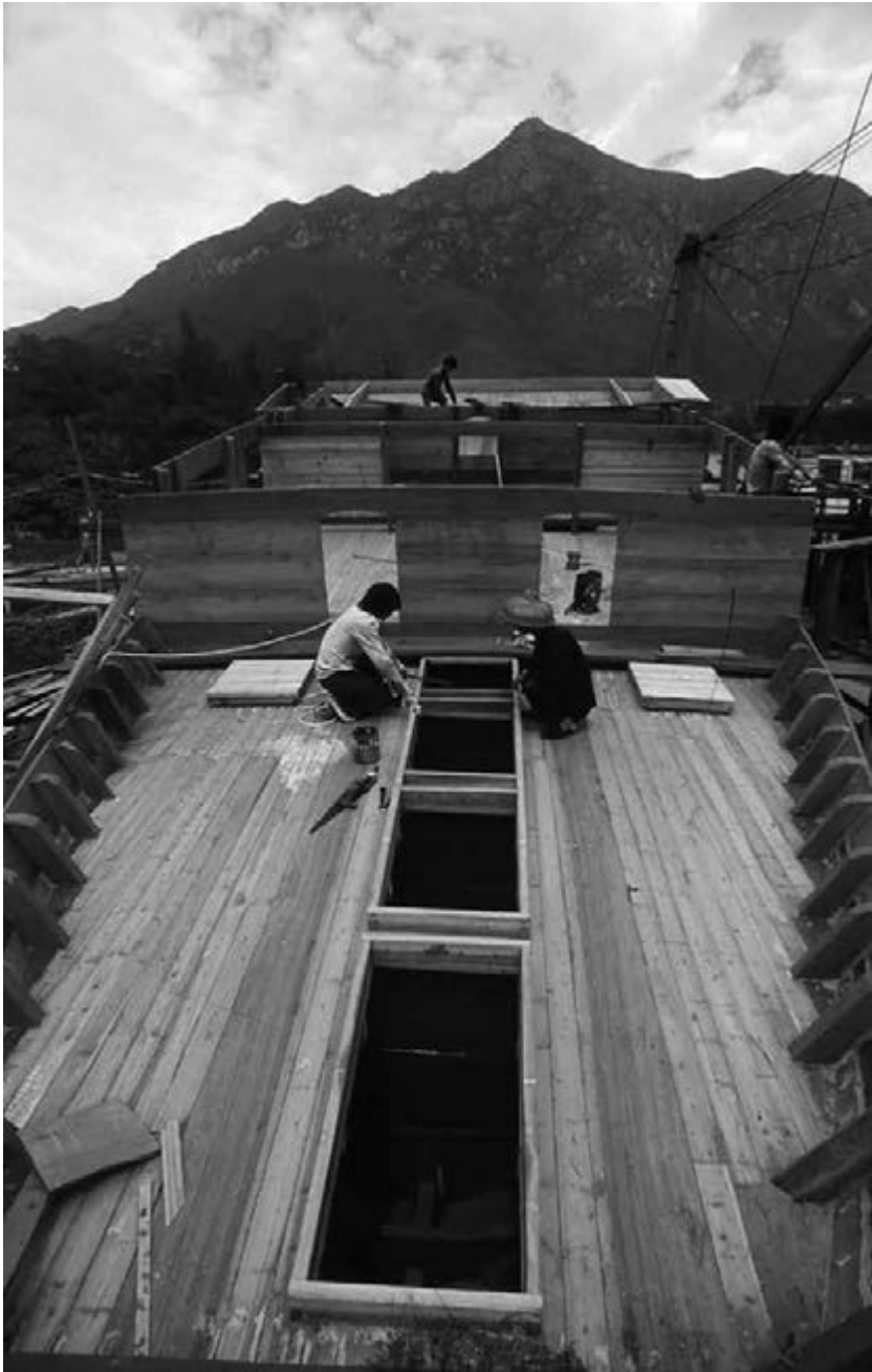
Figure 8 Compartments within the hull construction
