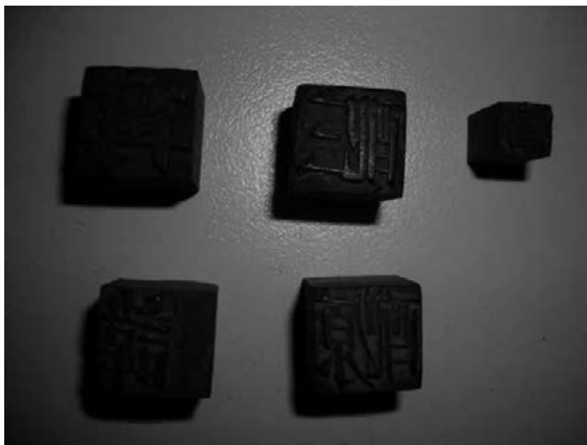
Figure 23 Individual wooden movable types in different sizes at the Gutenberg Museum, Mainz, dating about 1860
