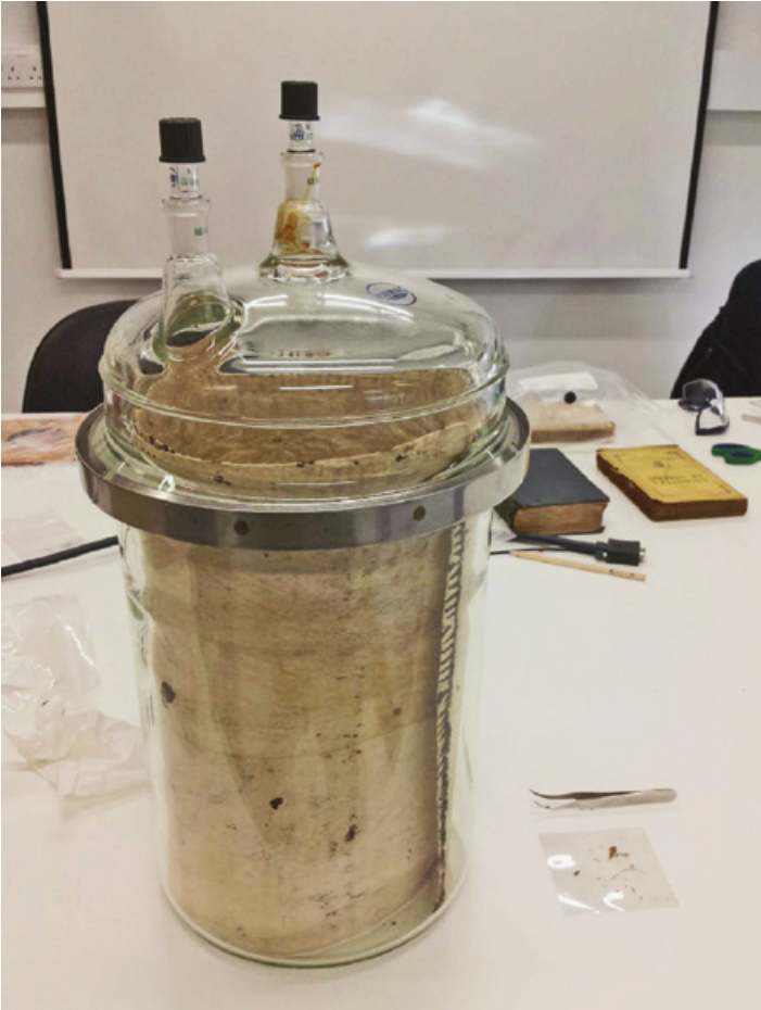
Figure 17 Barkcloth being measured for emissions at the UCL Institute of Sustainable Heritage. Photograph by Haidy Geismar.
