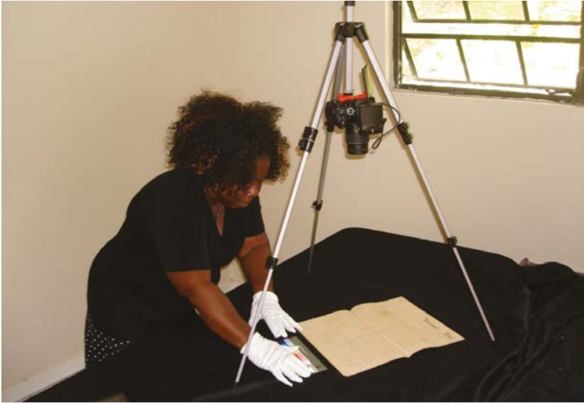
Figure 19. EAP769, Digitising using a tripod with camera attached to reversed centre column in Montserrat. Photo © Nigel Sadler, CC BY 4.0.
