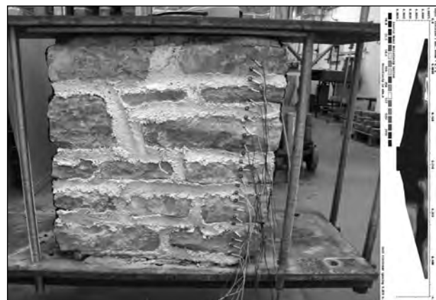
Figure 13. Test wall of Blue Lias constructed at UCL with probes attached (left), ERT result (right).
