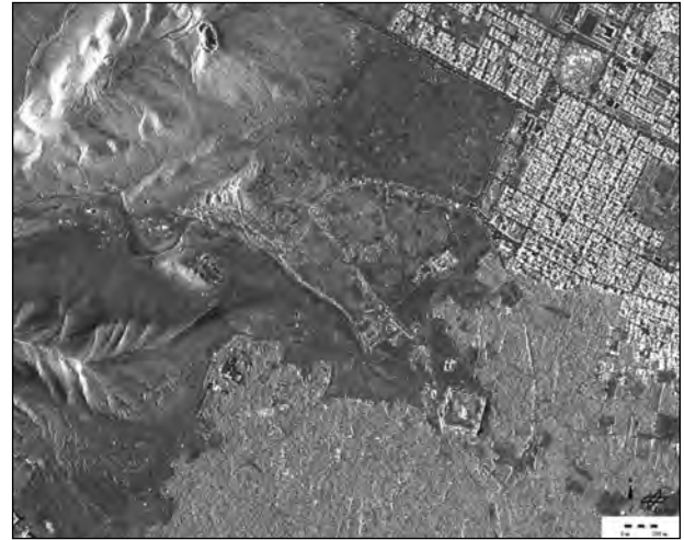
Figure 6. Radargram of TerraSAR-X in the area of the ancient Palmyra. Especially upstanding structures can be distinguished very well, but even parts of the buried archaeology are detectable. Data take: 28. February 2011, Horizontal polarisation, Spatially enhanced mode, Resolution: 1 – 2 m.
