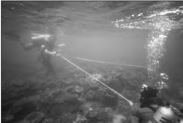
Figure 13. Simple trilateration on a wreck site using tape measures.
