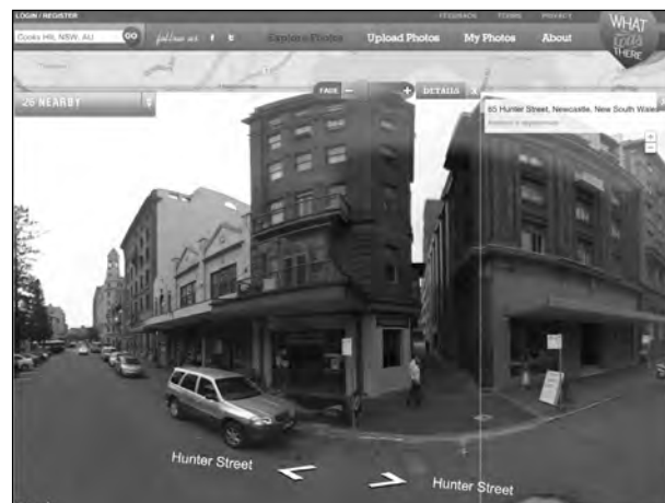
Figure 6. Streetscape, through Google Maps of Westminster Hotel. The body of the building still exists. Some of the Victorian detail has been stripped away with the modernisation of the building over the years and a further three floors added.
