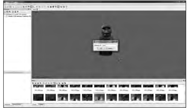
Figure 7. Defining measurement between two selected points to scale the photogrammetry model in AgiSoft Photoscan (Photo: James Miles).
