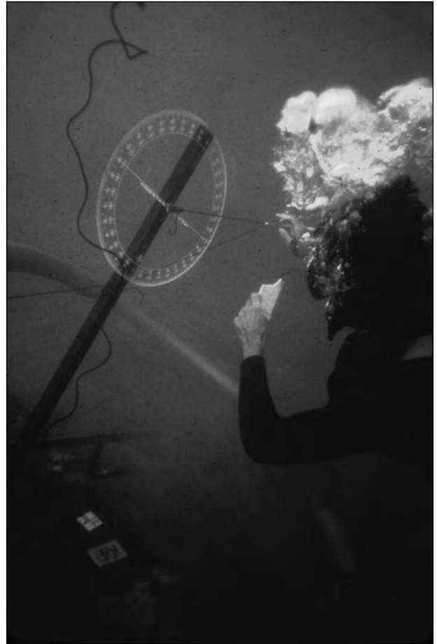
Figure 14. A simple angle measuring device being used to record the hull of a shipwreck.
