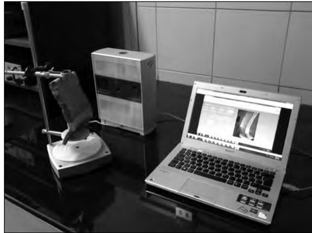
Figure 2. The scanning system: a NextEngine laser scanner connected to a computer and a rotatable support holding a ceramic fragment.
