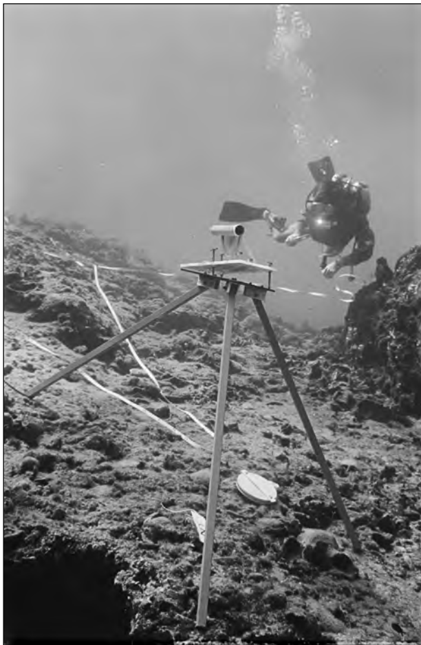
Figure 15. A simple underwater theodolite being used to record a site.
