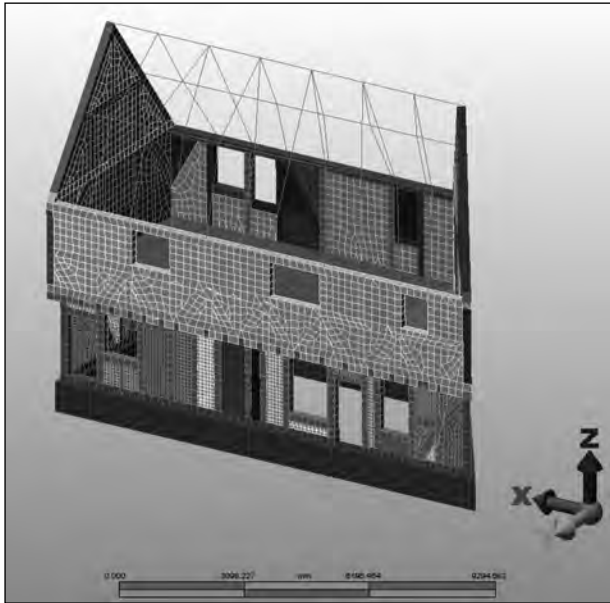
Figure 18. Finite Element model of Mill bank showing the division of the model into adjoining cells.
