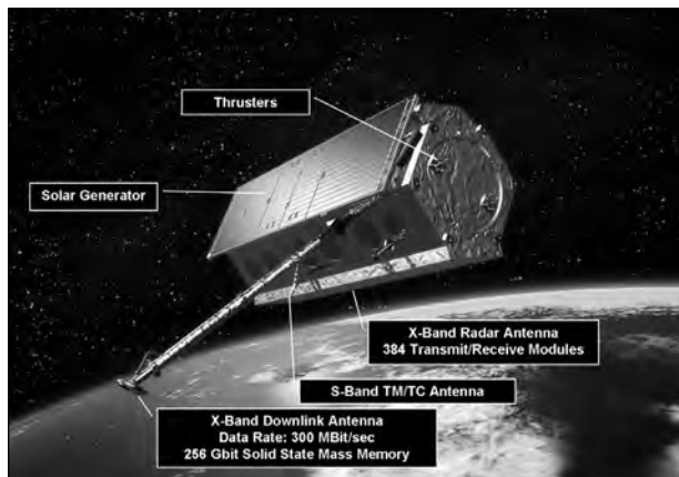
Figure 2. Artist view of the TerraSAR-X satellite. Note the solar generator (upper left), the boom with the X-Band downlink antenna (lower left) and the X-band radar antenna (lower right).
