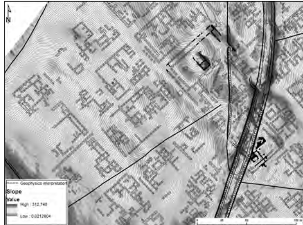
Figure 2. A high resolution DTM obtained by way of DGPS measurements on the Roman town-site of Ammaia (Portugal) was crucial for the mapping and interpretation of geophysics data (elaboration E. Paliou and V. Mayoral).
