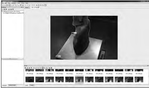
Figure 6. Photogrammetry scaling tool within AgiSoft Photoscan (Photo: James Miles).
