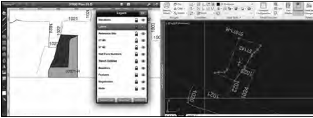
Figure 8. SU 57142 in both the TouchDraw (™) interface on the tablet (left) and AutoCAD (™) interface on the desktop (right).
