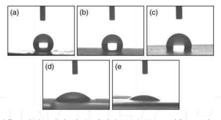
Figure 3. Photographs of water droplets taken immediately after contacting (a) non-treated, (b,c) oxygen plasma-treated and (d,e) ammonia plasma-treated PLGA nanofibers. Treatment time was varied from (b,d) 30 to (c,e) 180 s [128].
