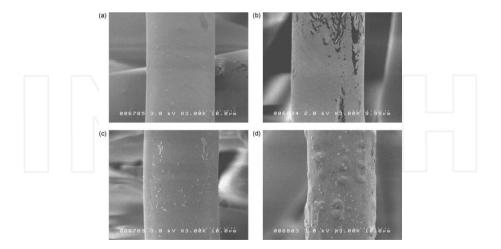
Figure 1. SEM micrographs (3000×) of the (a) plasma modified nonwoven, (b) AAc coated nonwoven, (c) PP-g-collagen nonwoven, and (d) PP-g-collagen-g-PNIPAAm nonwoven [126].
