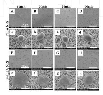
**Figure 4.** SEM images of pMSCs on Plasma treated PLLA nanofibers (NFS) and pristine PLLA NFS. (A–D) pMSCs on PLLA NFS after cultured for 10 min, 20 min, 30 min,60 min, respectively; (E–H) pMSCs on P-PLLA NFS after cultured for 10 min, 20 min, 30 min,60 min, respectively; (a–h) higher magnification for (A–H) [129].
