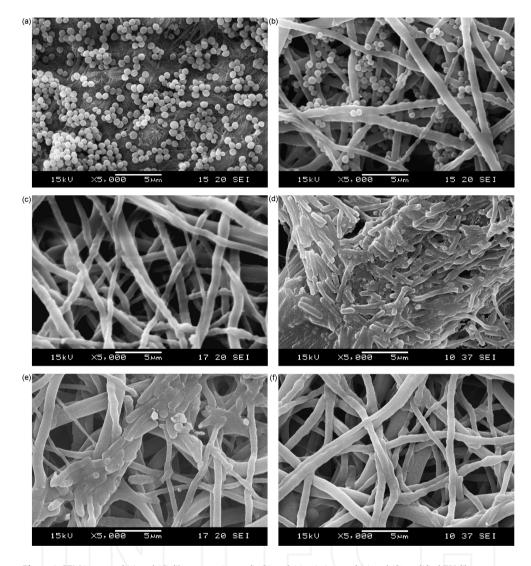
Figure 2. SEM images of (a) and (d) filter paper (control), (b) and (e) pristine, and (c) and (f) modified PU fibrous membranes after immersed in PBS suspension of (a)-(c) S. Aureus, or (d)-(f) E. Coli at 107 cells/mL for 4 h. PU fibrous membranes were electrospun from 10% (w/v) solutions in THF and DMF (1:1, v/v) [127].
