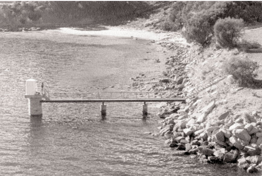
Figure 2.5 Tide gauge at Spring Bay, Tasmania, part of the ‘Seaframe’ set of precision gauges collecting data for the National Tidal Facility
