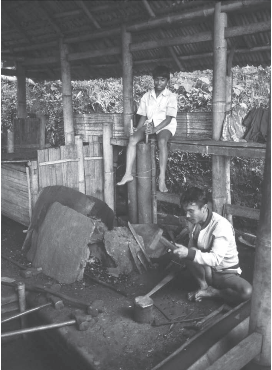
A blacksmith's forge on the slopes of Mount Sesean, 1983. The boy sitting above is working the bamboo bellows. The creator deity Puang Matua is described in ritual poetry as creating the first human ancestor in his forge with the 'twin bellows' ( sauan sibarrung ), just as seen here.
