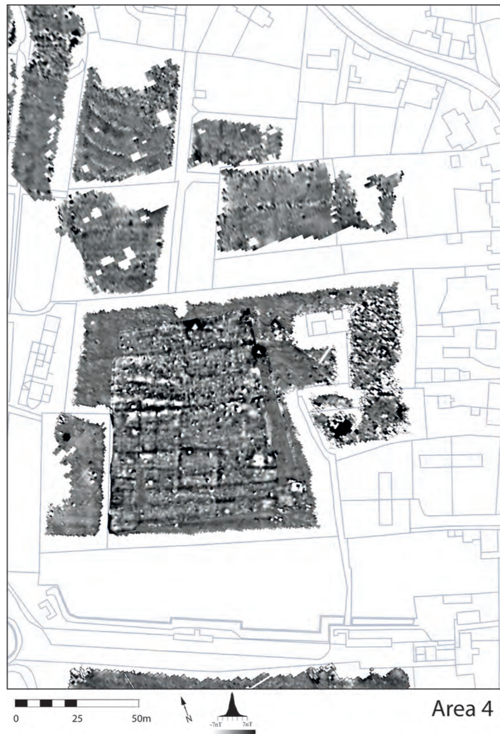
Fig 3.15 Area 4: results of the gradiometry survey in relation to modern topography. For the location, see fig 3.3. Scale 1:1500. Drawing: Rose Ferraby. © Crown copyright and database rights 2018 Ordnance Survey (100025252)
