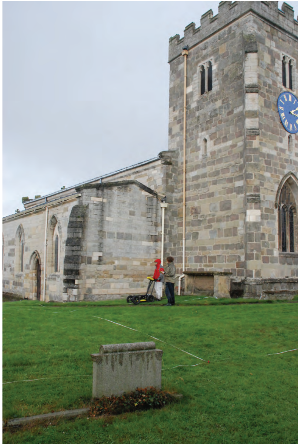
Fig 3.2 Rose Ferraby and Jess Ogden undertaking GPR survey on site using a Noggin Plus System with rugged terrain cart and 500 MHz antenna. Photograph: Martin Millett
