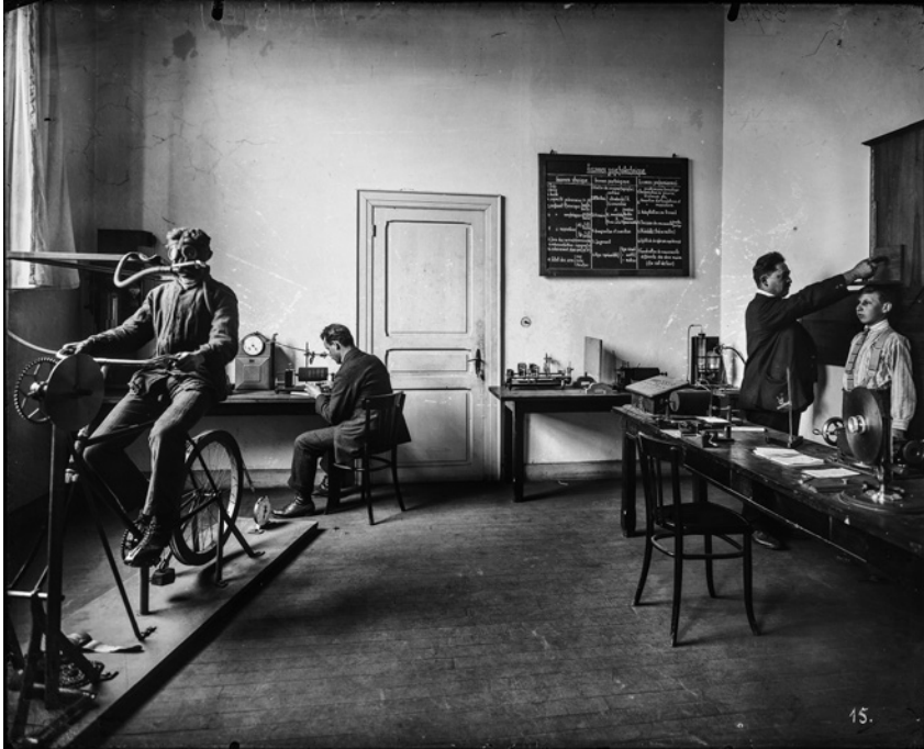
FIGURE 5.3 Psychophysiological laboratory at the Institut Emile Metz: On the left, a young man is training on an ergometric bicycle. In the background, on the right, one can see three cylindrical recorders and the mercury manometer. Digital positive from glass plate negative.
