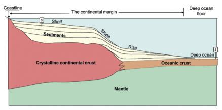
FIGURE 1.1 Profile showing a cross section of the elements of the general topography of the seabed extending from the coastline to the deep ocean floor
