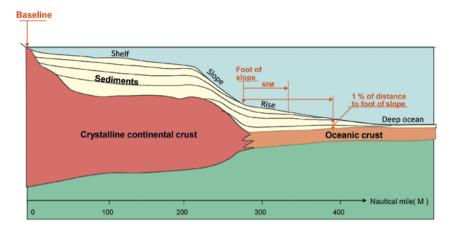
FIGURE 4.1 Schematic profile of the continental margin with geological terms in black and delineation terms of Article 76 in red. According to Article 76, the outer edge of the continental margin is to be set at a distance of either 60 nm from the foot of the slope (the Hedberg Rule) or at a location where the sediment thickness is not less than 1% of the distance to the floor of the slope (the Gardiner Rule)
