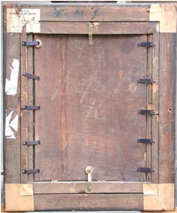
Figure 8 Inappropriate framing causing fracture in panel (Ray Marchant)
