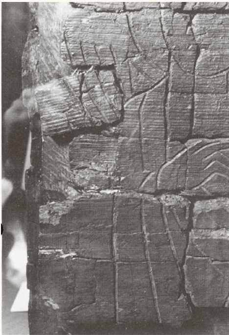
Figure 5 A fragment of degraded wood of St Cuthbert's coffin adhered with PVAC slumped over 30 years, due to the low T_g of the polymer. (Cronyn and Horie 1985)
