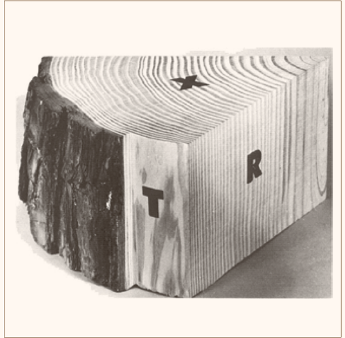
Figure 2 Wood sections, X: cross section, R: radial, T: tangential (Wolfgang Gard)
